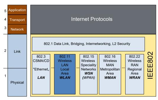
Specifies only Physical and Link Layer. Complete set of standards for carrying IP
