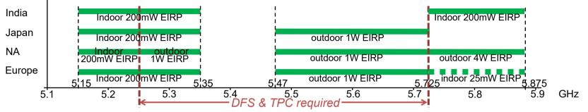
• Dynamic Frequency Selection (DFS) and Transmission Power Control (TPC) are required for most of the 5 GHz spectrum to protect primary users (e.g. weather radars)
