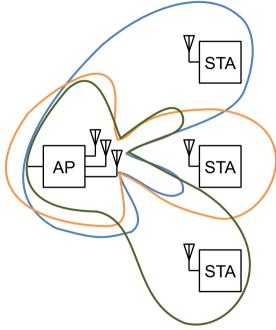
MU- MIMO with combination of Beamforming and Null Steering
