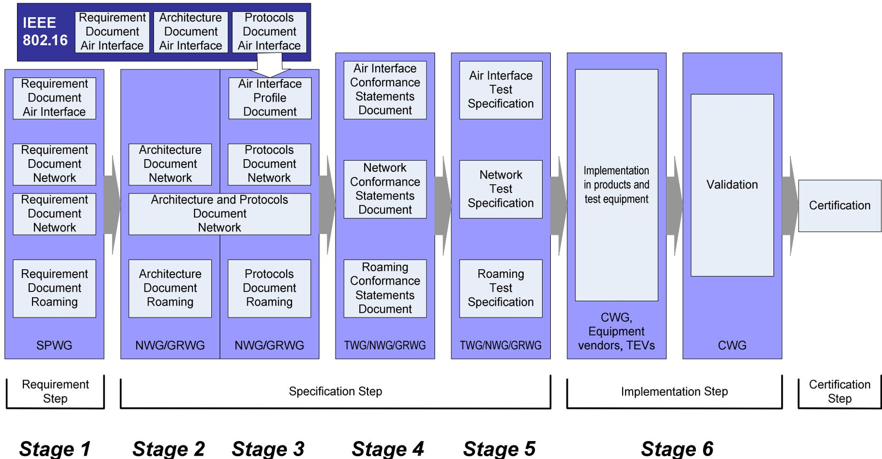
WiMAX Forum Standardization extended the legacy 3-stage process to 6 stages to establish certified interoperability in Mobile WiMAX.
